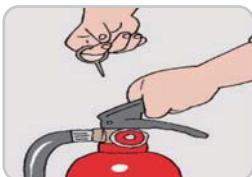
Remove the safety pin from the fire extinguisher (hold the top lever with the hand when doing so).
