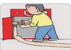
Slowly rotate the fire hydrant valve counterclockwise to loosen it.
